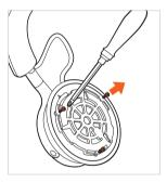
Loosen the six screws inside the ear cup with a cross-head screwdriver (PH0X40).
