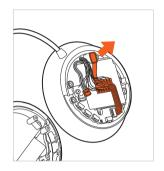
Loosen the adhesive connection under the battery with a suitable flat tool and pull the battery out under the conductor tracks.
