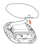
Disconnect the cables leading to the battery.
