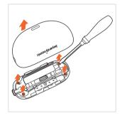
Loosen the two screws on the circuit board.
