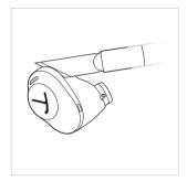
Loosen the plug connection on the side. Pinch off the heads of the three plastic pins.
