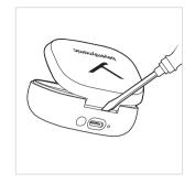
Loosen the insert and remove the lower part of the housing.
