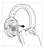
Carefully remove the baffle.
