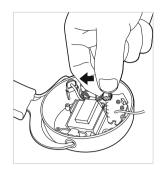
▶ Grab the strap under the battery with a small pair of needle-nosed pliers and turn it until you can pull out the adhesive pad under the battery. The battery comes off from the bottom and can be removed.
