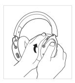
Loosen the three screws of the baffle on the right-hand side of the headphones using a suitable screwdriver.
